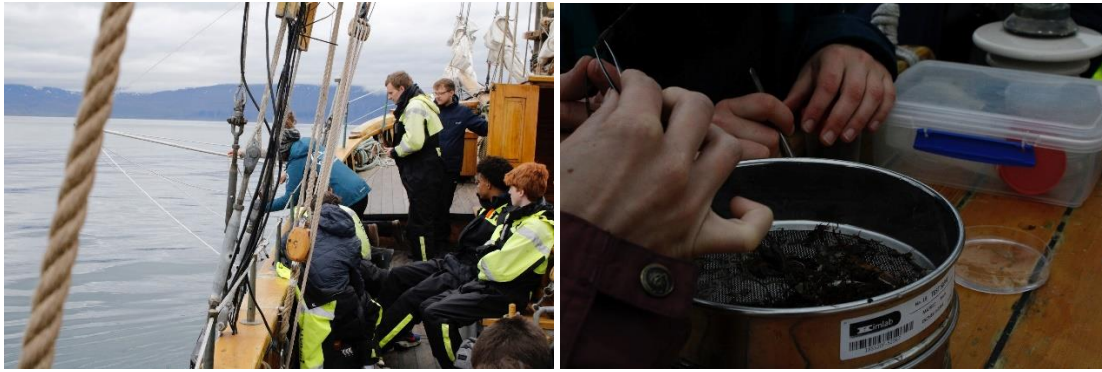
Figures 11-12: Microplastic trawl deployed by researchers and samples filtered, participants observe ©Gyde Rudolph
